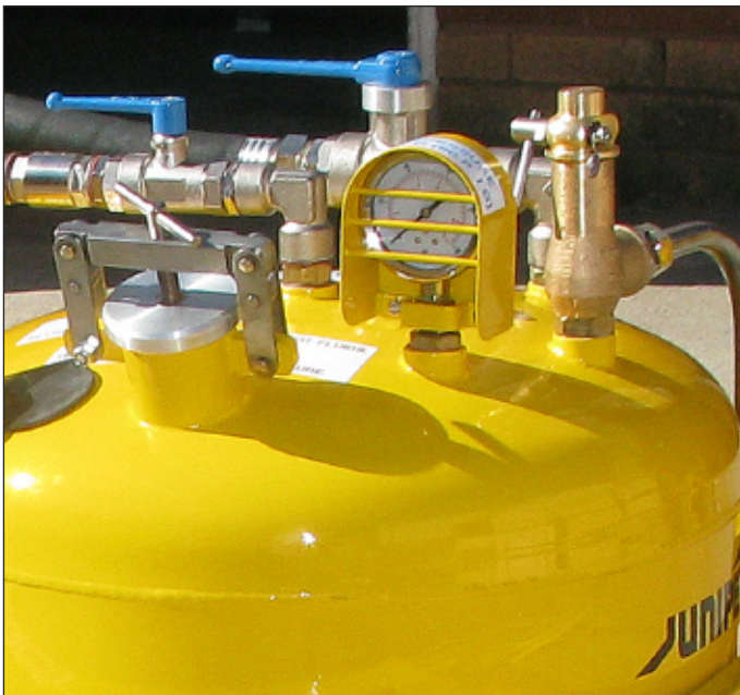
Pressure gauge positioned correctly on the tank.
